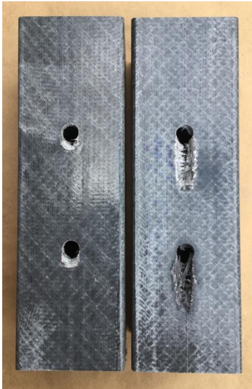
4% ELONGATION POINT FAILURE AT >4% LOAD
